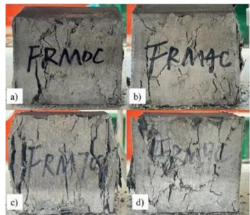
FIGURE 6 CUBE COMPRESSIVE FAILURE PATTERN OF FIBER REINFORCED CONCRETE WITH DIFFERENT MPCM LEVEL: A) 0%, B) 4%, C) 7%, D) 9%
