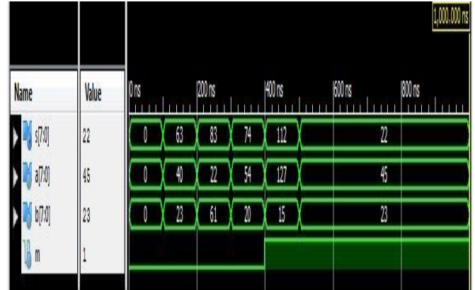
Figure 8: Result in test bench Conventional 8 bit full adder/Subtractor
